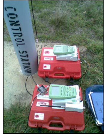
Figure 2: GNSS receivers with antenna cable splitter
