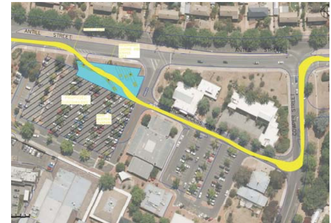
Figure 11: Services vehicle 'swept' path
